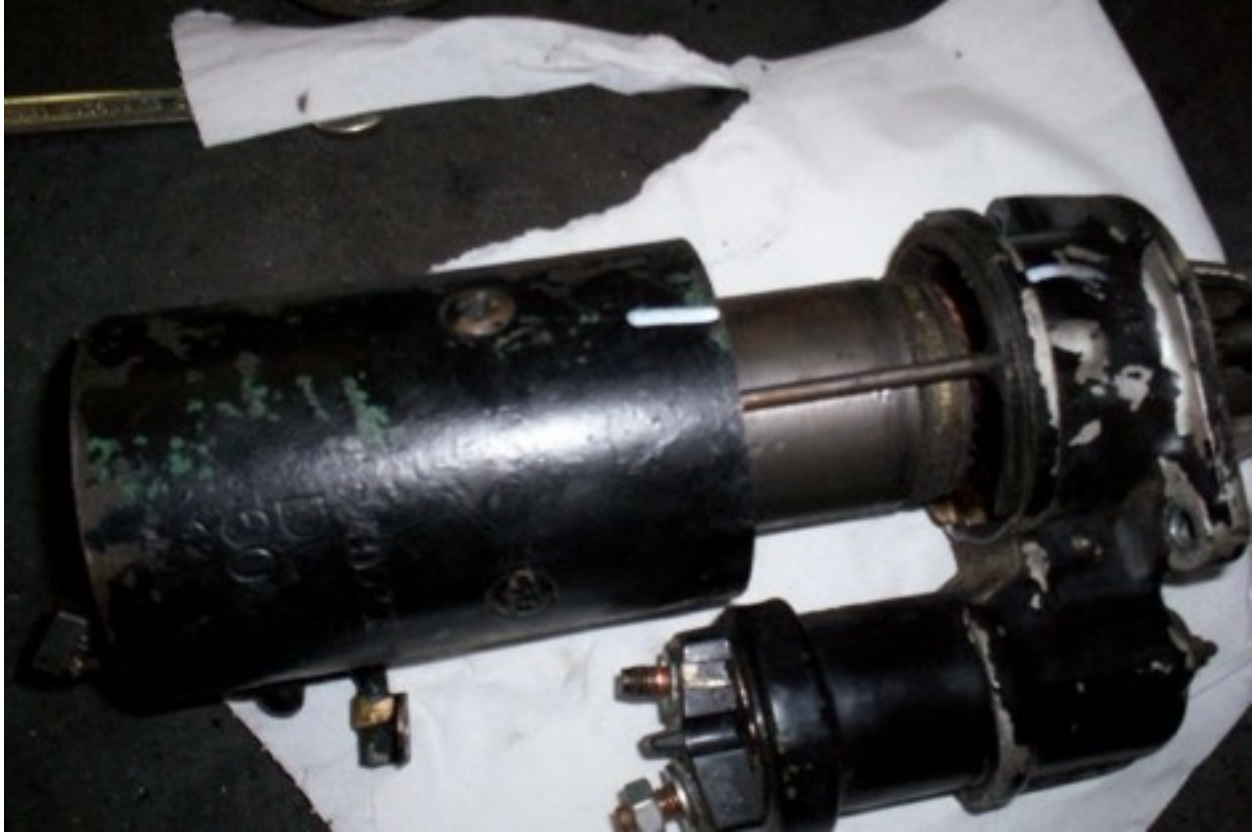
Removing the spindle from the solenoid fork using a pin hook.
