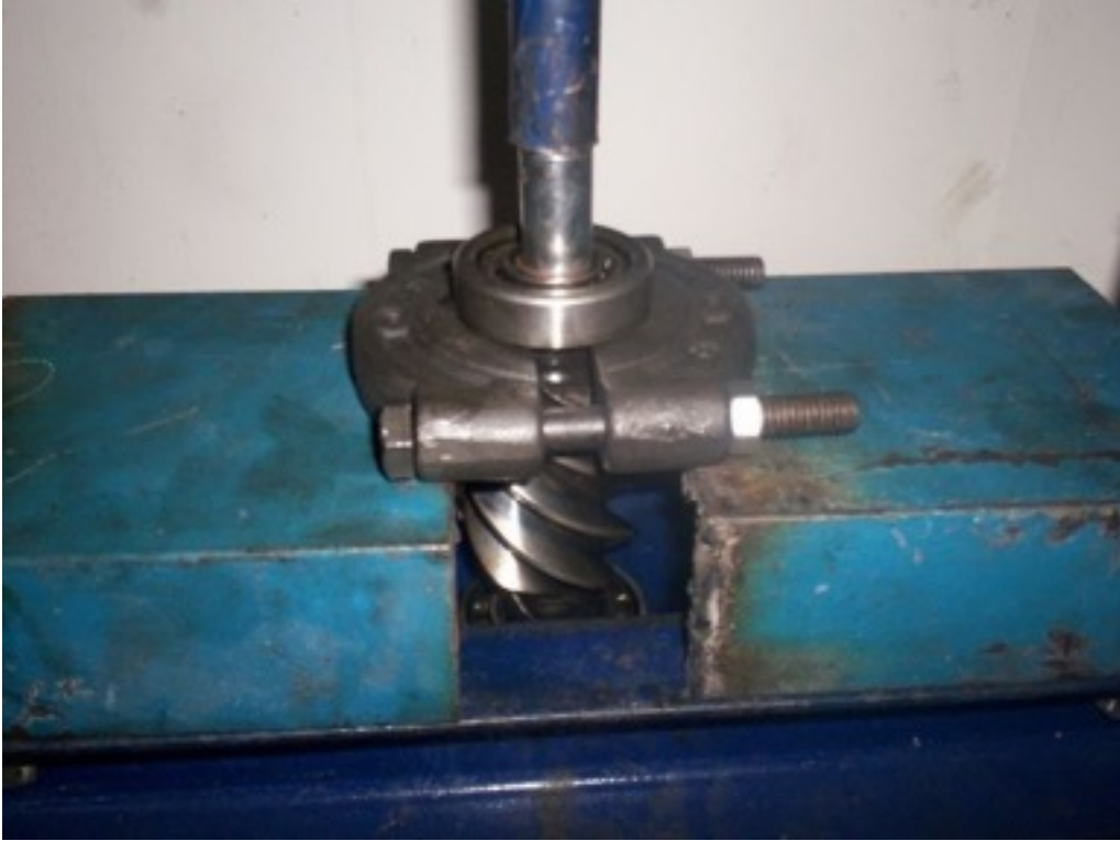
Removing the front and rear bearings from the screw
