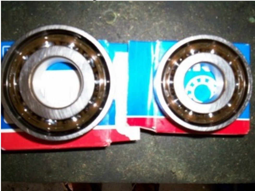
Face of the two bearings external sides of the screw.
